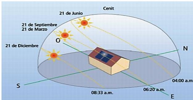
Figure 4 Cardinal position of the sun according to the date
